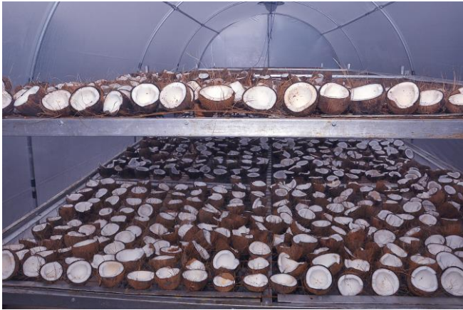
Fig. 9 Drying of Coconuts Inside the Solar Tunnel Dryer
