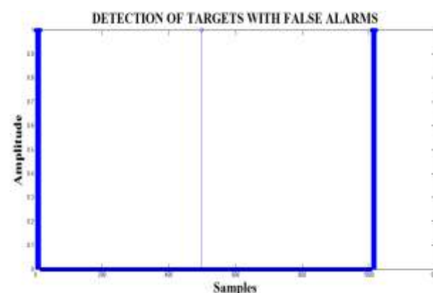
Figure 5. CFAR Output in the Presence of False Alarms
