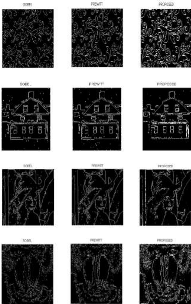
Fig. 7: Results of our algorithm compared with Sobel and Prewitt corrupted with salt and pepper noise
