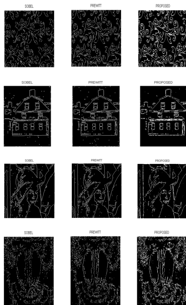
Fig. 7: Results of our algorithm compared with Sobel and Prewitt corrupted with salt and pepper noise
