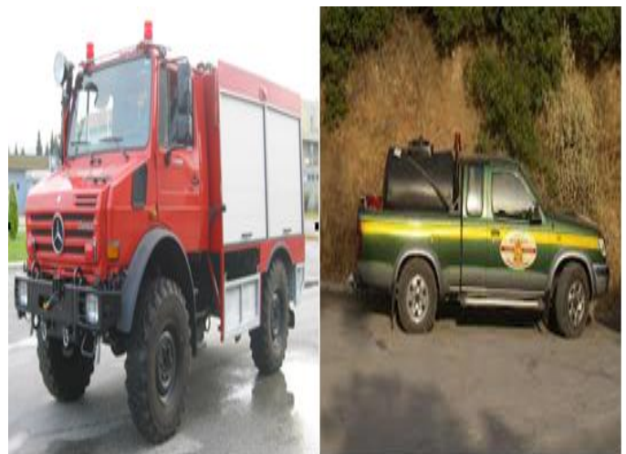
Fig. 7, Typical firefighting vehicle (UNIMOG of ELBO) and tank in agile van 4x4
