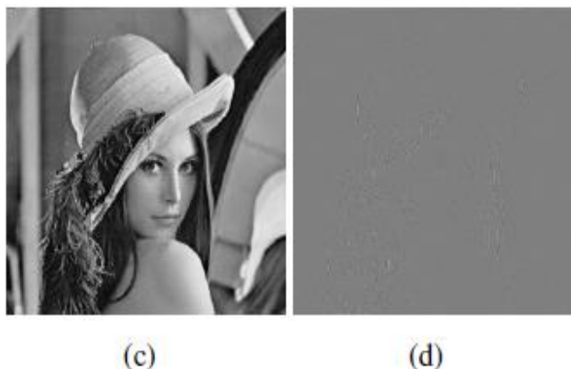
Figure 3 (c) low-pass subband and (d) high-pass subband from the proposed lifting technique
