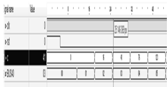
Fig-14 Output waveform for digit serial adder using transpose and MCM
