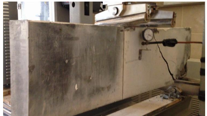
Fig. 5 Failure pattern of ferrocement deep beam BH7.
