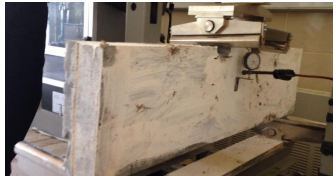
Fig. 2 The erection of a beam inside the loading frame
