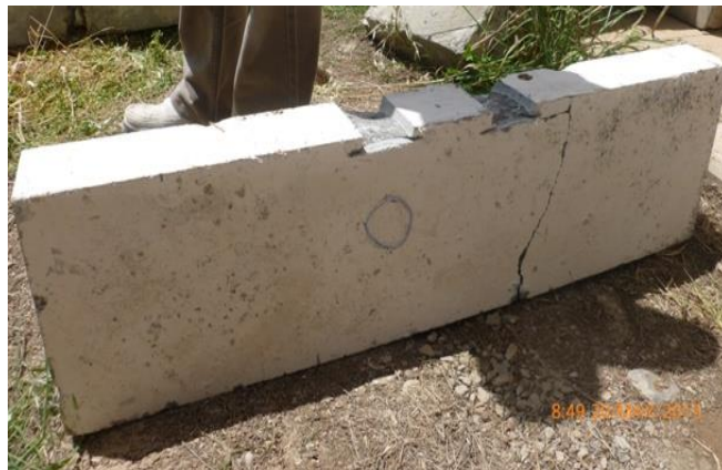
Fig. 4 Failure pattern of ferrocement deep beam B0.
