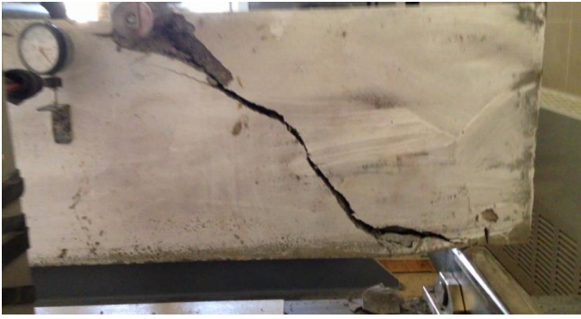
Fig. 8 Failure pattern of ferrocement deep beam BN12
