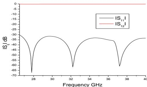
Figure 7: Transmission coefficients  $S_{21}$  and reflection  $S_{11}$  of the RSIW
