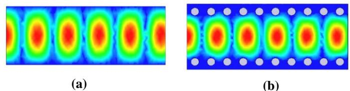
Figure 4: Electric field distribution of the  $TE_{10}$  mode in the equivalent rectangular waveguide (a) and RSIW (b) at the frequency  $f = 33\text{GHz}$
