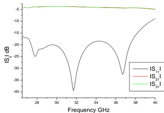
Figure 15: Parameters  $S_{ij}$  in the power divider with inductive cylinder
