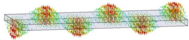
Figure 2: Electric field of  $TE_{10}$  mode rectangular waveguide equivalent,  $W_{eq}=4.795\text{mm}$ ,  $h=0.508\text{mm}$ ,  $\epsilon_r = 2.2$  at frequency  $f = 33\text{GHz}$
