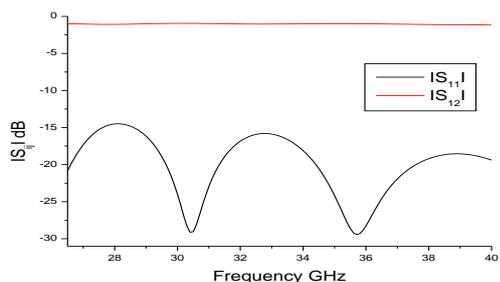
Figure 8: Transmission coefficients  $S_{21}$  and reflection  $S_{11}$  of RSIW with taper
