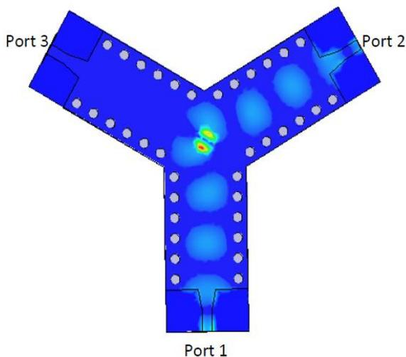
Figure 17 : Electric field distribution of the TE<sub>10</sub> mode of the RSIW circulator at f = 33.7 GHz
