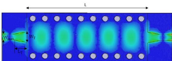
Figure 6: Electric field distribution of  $TE_{10}$  mode at  $f = 33$  GHz in the matched RSIW
