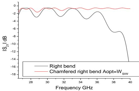
Figure 11: Comparing transmission coefficient  $S_{21}$
