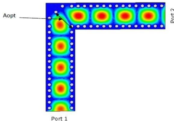
Figure 10: Plot of the  $TE_{10}$  electric field magnitude of a RSIW chamfered bend  $A_{opt}=W_{SIW}$  at  $f=28$ GHz
