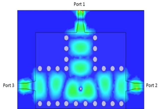
Figure 14: Electric field distribution of the  $TE_{10}$  mode at  $f = 31.5\text{GHz}$  in the power divider with inductive cylinder
