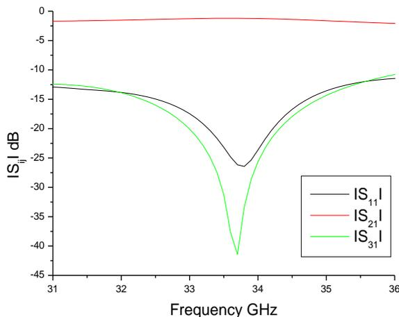
Figure 18: Parameters S<sub>ij</sub> of RSIW circulator
