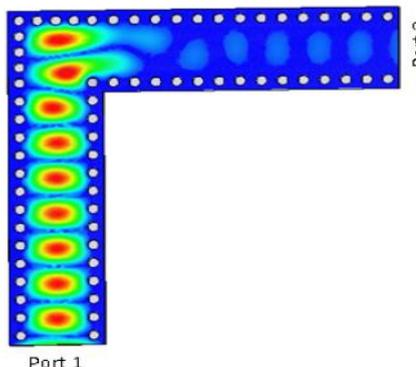
Figure 9: Simulation of the  $TE_{10}$  electric field magnitude of a right bend at  $f=40$ GHz
