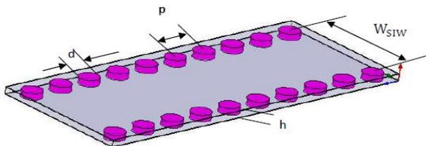
Figure 1: rectangular wave guide integrated into a substrate RSIW
