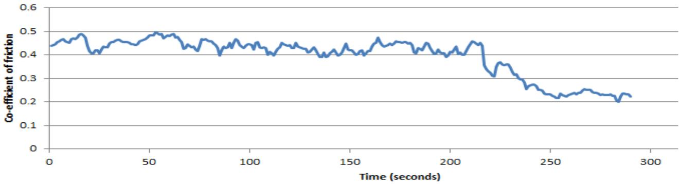
Fig. 2(a) Dependency of co-efficient of friction with time. Material; Casehardened carbon steel (uncoated)
