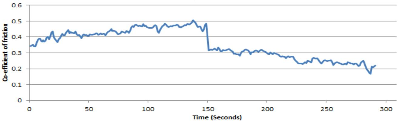
Fig. 2(d) Dependency of co-efficient of friction with time. Material; Casehardened carbon steel (Zinc coated)
