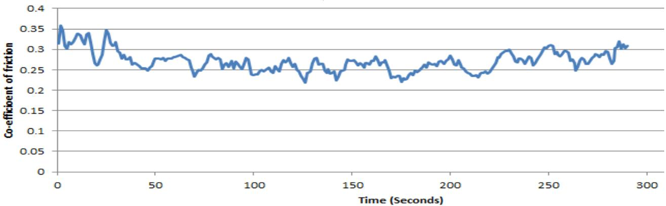
Fig. 2(c) Dependency of co-efficient of friction with time. Material; Casehardened carbon steel (Tin coated)
