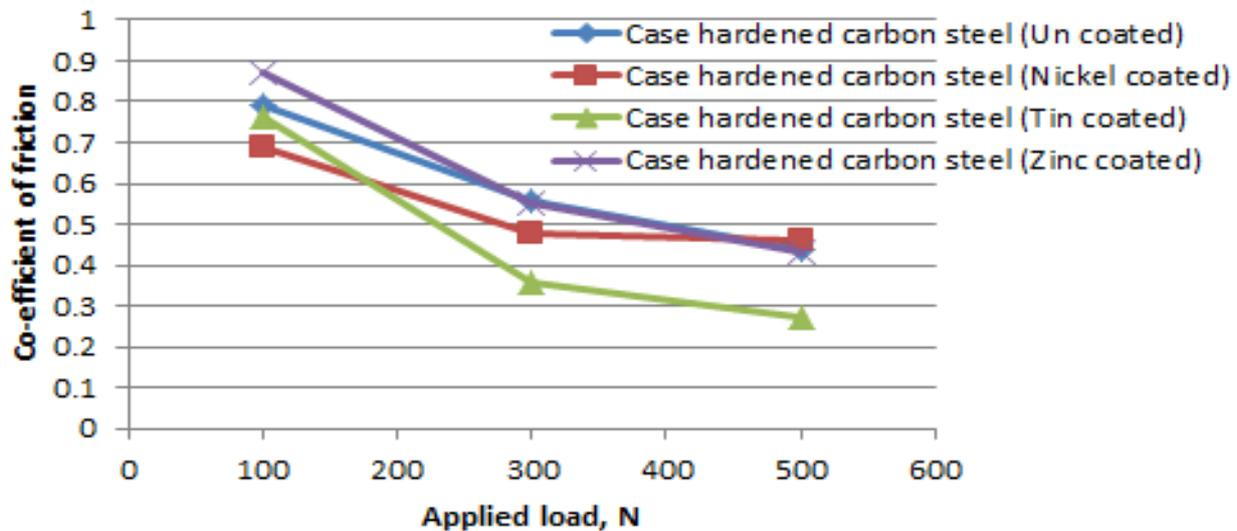
**Fig.3 Co-efficient of friction with applied load for casehardened carbon steel balls (uncoated) and coated with nickel (Ni), tin (Sn) and zinc (Zn).**
