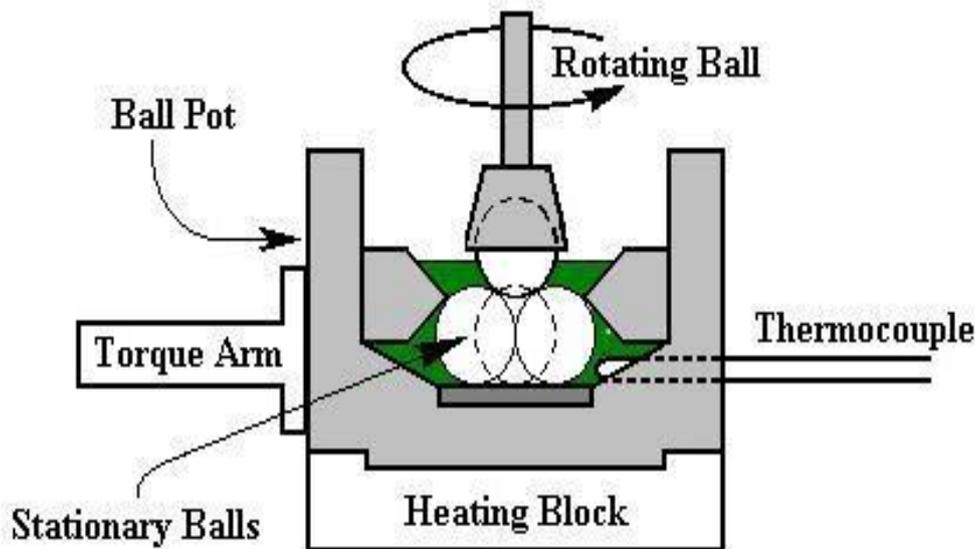
**Fig.1 Schematic Diagram of Four Ball Test Rig**
