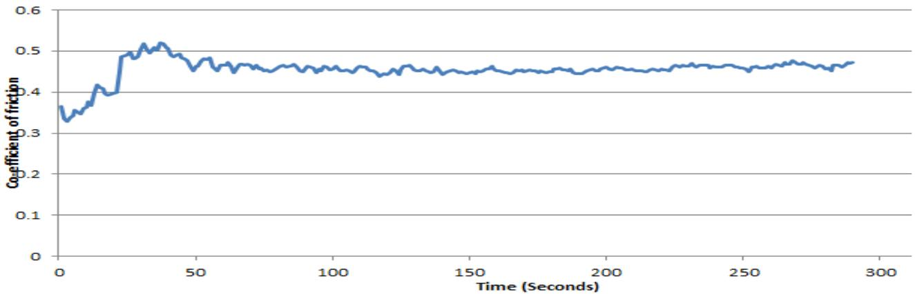
Fig. 2 (b) Dependency of co-efficient of friction with time. Material; Casehardened carbon steel (Nickel coated)
