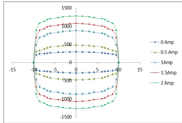
Fig 6: Damping Force Vs. Displacement (MRF3)
