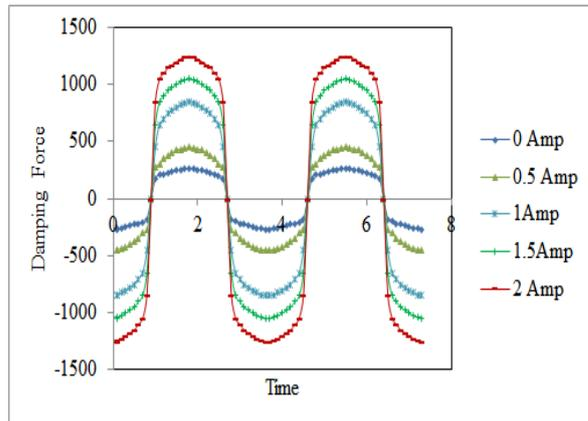
Fig 7: Damping Force Vs. Time (MR1)
