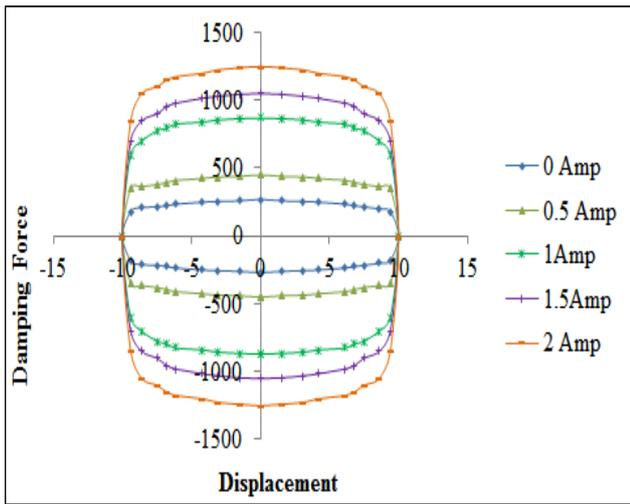
Fig 4: Damping Force Vs. Displacement (MR1)
