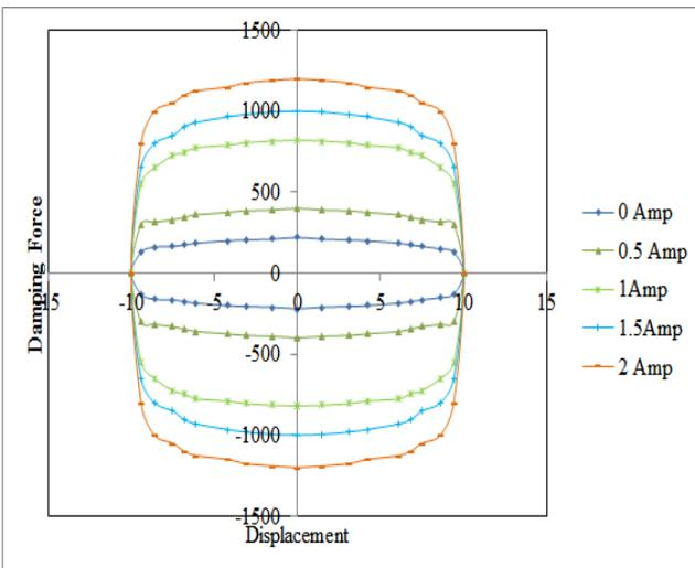
Fig 5: Damping Force Vs. Displacement (MR2)
