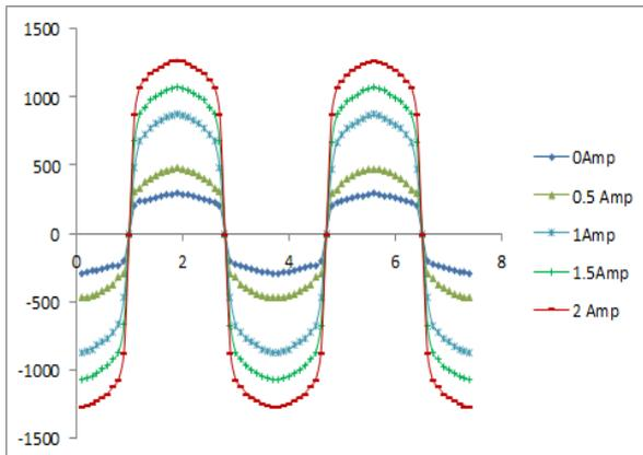
Fig 9: Damping Force Vs. Time (MR3)
