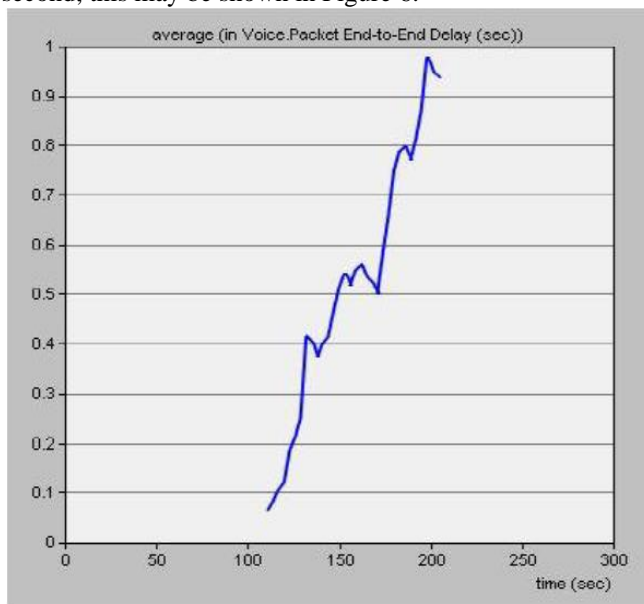
Figure 6: WiFi base line voice-packet end to end delay.
