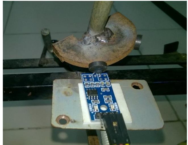
Figure 3. Hall effect sensing mechanism
