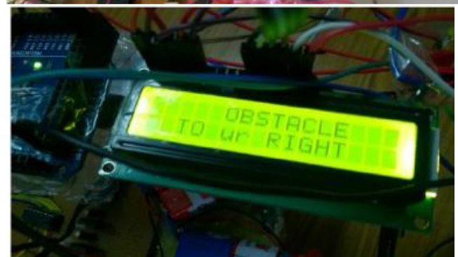
Figure 7. LCD Alert of Obstacle at the rear end
