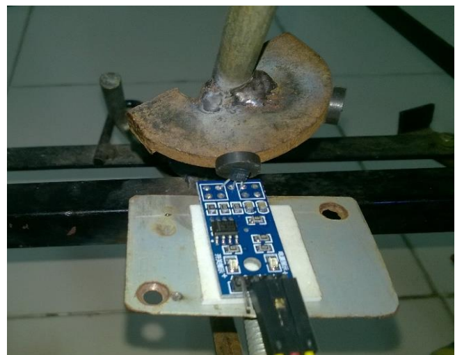
Figure 3. Hall effect sensing mechanism
