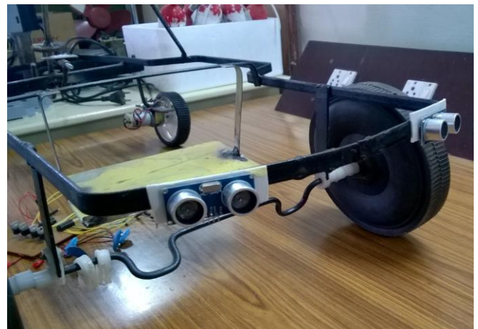
Figure 4. Rear end with Ultrasonic sensors fixed
