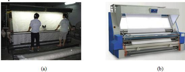
Figure 2: Shows the types of inspections (a) Manual and (b) Machine Automated
