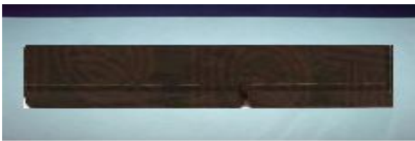
Figure 2 cryogenically treated En 19 steel specimen
