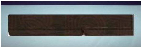
Figure 2 cryogenically treated En 19 steel specimen
