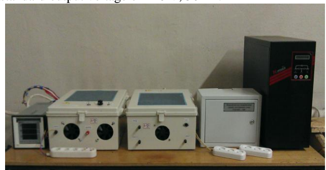
Fig. 3. A set of equipment for electrical energy transmission in resonant mode
