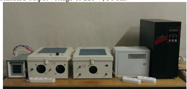
Fig. 3. A set of equipment for electrical energy transmission in resonant mode
