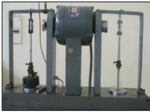
fig-2 fatigue testing machine
