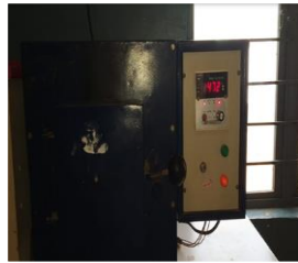
fig-3 Heating Furnace
