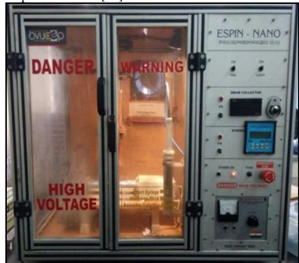
Figure 2: Electro spinning machine actual setup at BVDUCOEP
