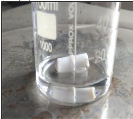
Figure 1: Before dissolving PAN in DMF (transparent colored solution)
