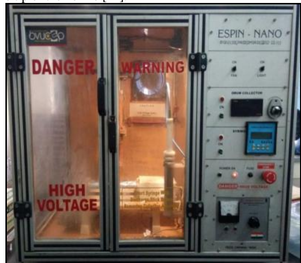
Figure 2: Electro spinning machine actual setup at BVDUCEP
