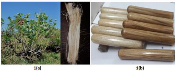
Fig 1.(a). Madar tree and fiber. (b). Nano-Khorasan based Madar fiber composites for turning experiments.
