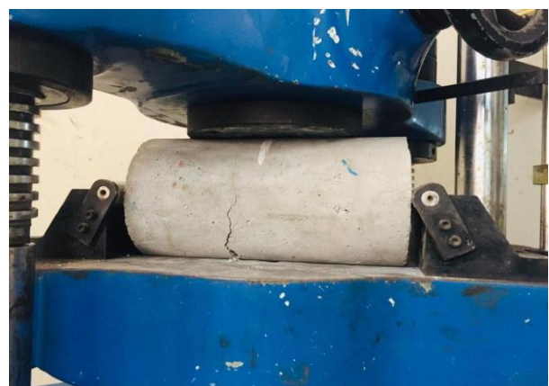
Figure 3: Split tensile strength test by using UTM
