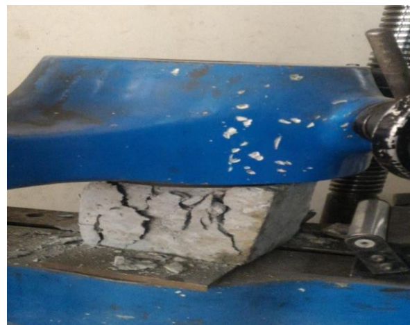
Figure 1: Compression test by using UTM
