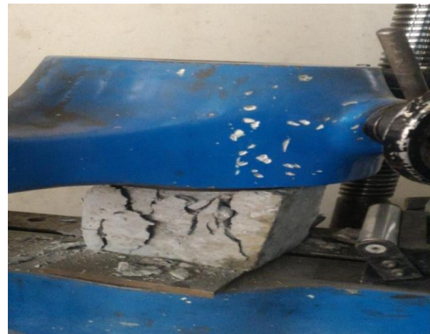
Figure 1: Compression test by using UTM
