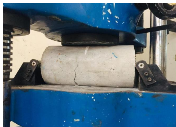
Figure 3: Split tensile strength test by using UTM
