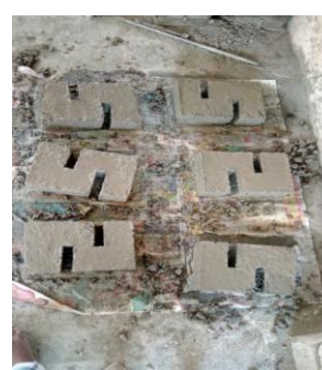
Fig.7: Double 'L' Shear Shear mould
