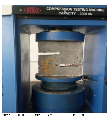
Fig.11: Testing of beam Shear
