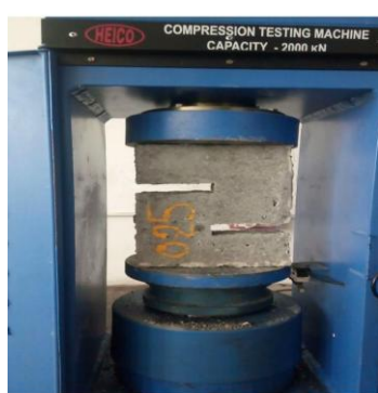
Fig.11: Testing of beam Shear
