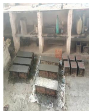
Fig. 5: Beam specimens after casting.
