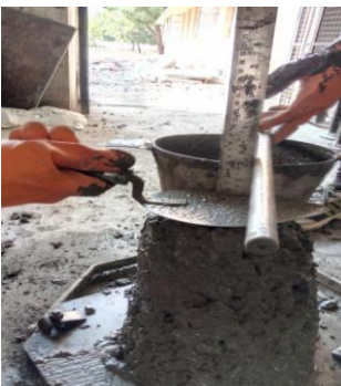
Fig. 9: True slump for 0% Admixture
