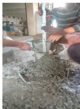
Fig.10: Collapse slump for 0.75% Admixture
