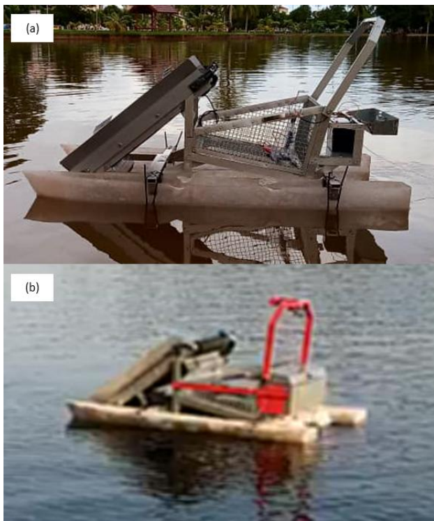
Fig. 4 Water displacement level of trash collector boat (a) Before loading (b) After full load
