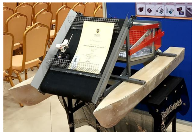
Fig. 3 Prototype of portable trash collector boat
