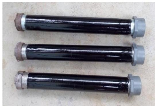
Fig.4 Anchor as per ASTM D7205
