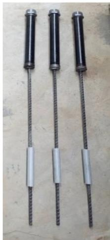
Fig.5 (a) BFRP bars (Ready for casting)
