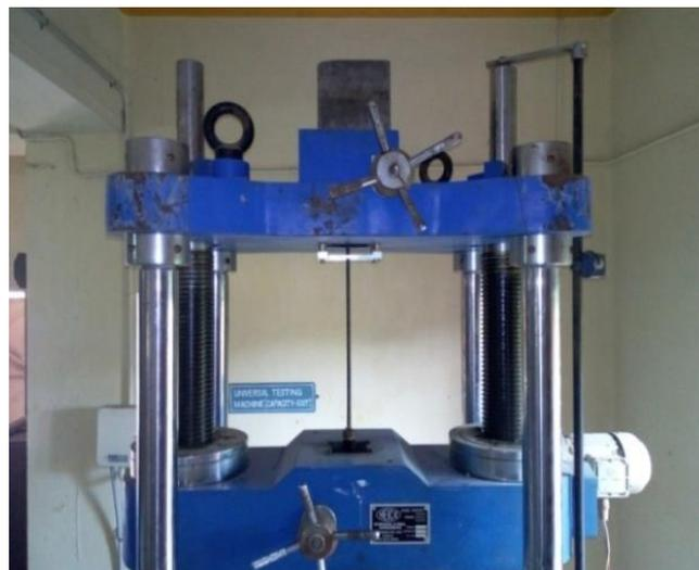
Fig. 6 (a) Pullout test setup
