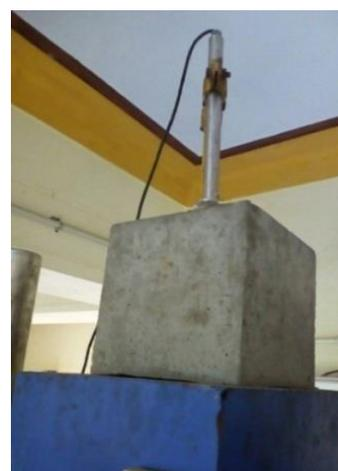
Fig.7. LVDT at Free end of BFRP bar
