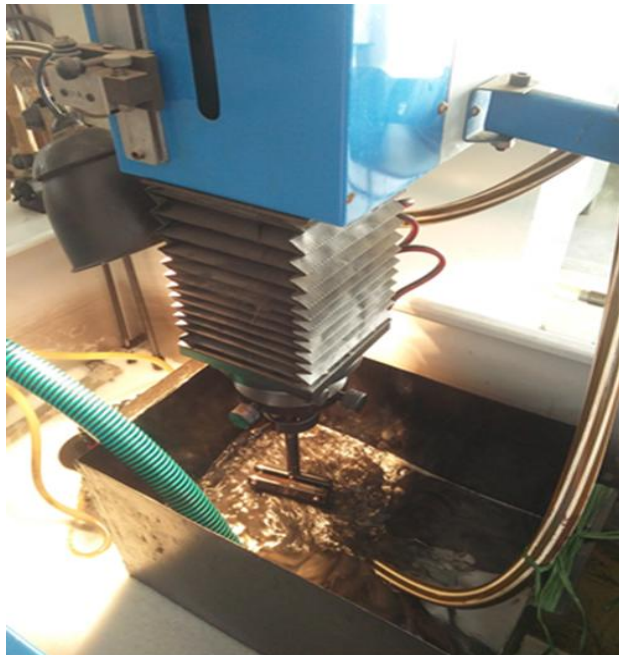
Fig. 1 An experimental setup for the EDM process
