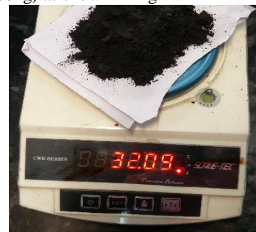
Fig. 2 Weight measurement of the powder particles
