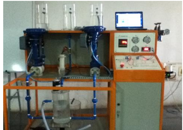
Fig.2. Hardware set up of the pH Neutralization plant
