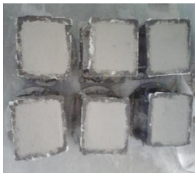
Figure. 1 The casted Cube specimen
