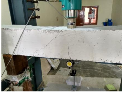
Figure. 5 Flexural strength test on Beam
