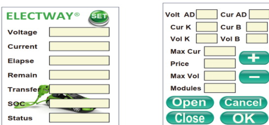
Fig. 2. HMI display screen of DC charging station of Electway
