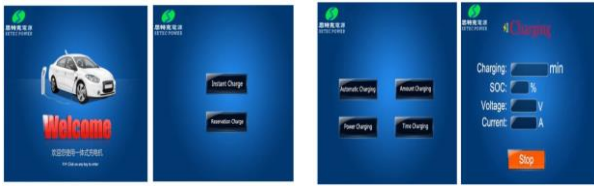
Fig. 1. HMI display screen of DC charging station of MassTech
