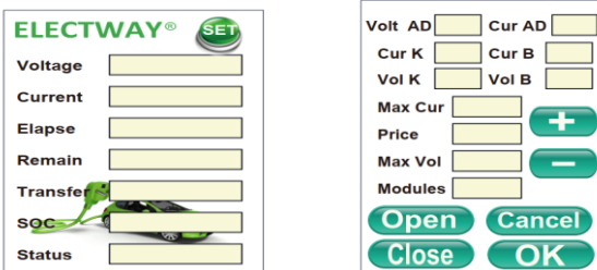
Fig. 2.HMI display screen of DC charging station of Electway
