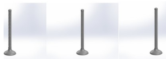
Fig2: Intake and Exhaust valve Pitch diameter 1mm,1.5mm, 0.2mm
