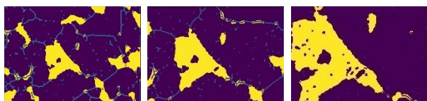
Fig.2: processed images corresponding to the original SEM images (row 1&2) at six different resolutions (500X to 5000X) obtained by Chan-Vese (row 3&4) algorithm.
