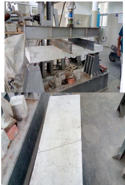
Figure 6.5 Testing of Slab Figure 6.6 Crack Pattern of Slab
