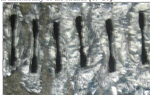
Fig. 1 Specimens For Tensile test
