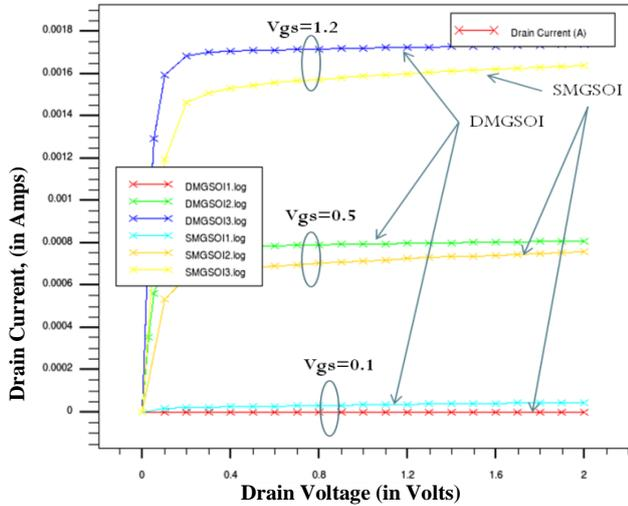
Figure 4 Drain current versus drain voltage
