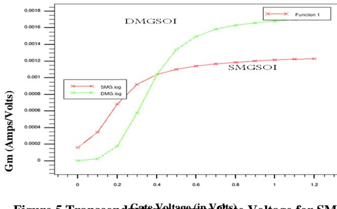
Figure 5 Transconductance versus Gate Voltage for SMG and DMG SOI MOSFET
