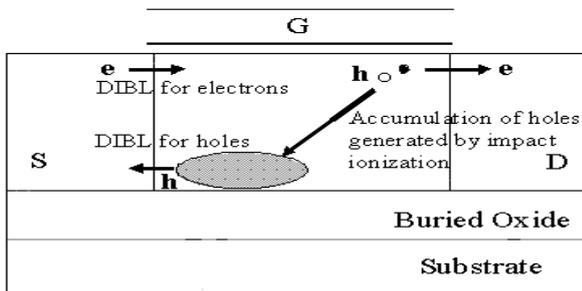
Figure 1. The mechanisms determining SCE in SOI MOSFETs [2]
