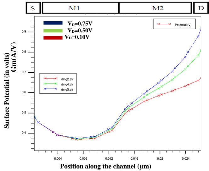
Figure 6 Surface potential profiles for DMG-SOI MOSFET at various drain voltage along the channel
