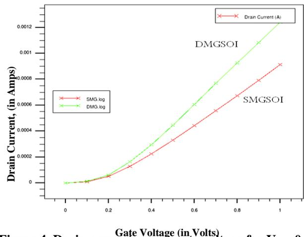
Figure 4. Drain current versus gate voltage for  $V_{Ds}=0.1$
