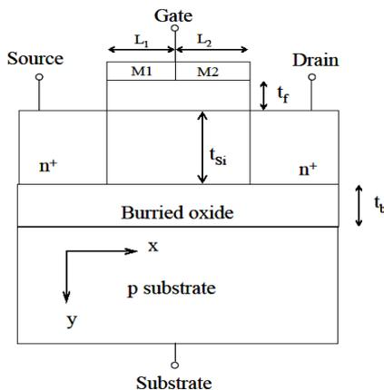
Figure 2. Cross-sectional Schematic of DMG-FD-SOI MOSFET
