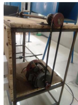
Fig.2. V Belt, two cone pulleys and single phase induction motor of \frac{1}{2} HP
