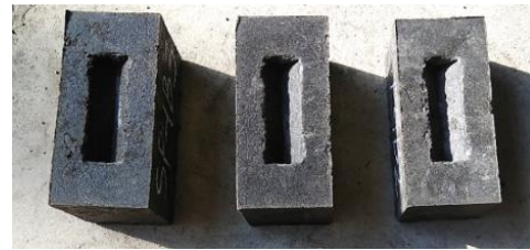
Figure 13 Visual Inspection of Bricks
