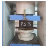
Figure 11 Compression Test Performed on Plastic Sand Brick [2]
