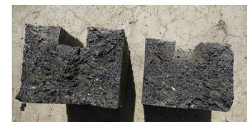
Figure 20 Broken Structure of Plastic- Iron Chips Bricks
