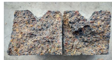
Figure 18 Broken Structure of Plastic -Moorum Brick
