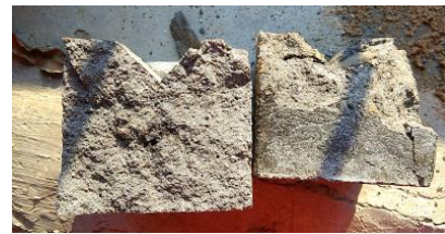
Figure 17 Broken Structure of Plastic Sand Brick
