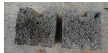
Figure 19 Broken Structure of Plastic -Quarry Dust Brick
