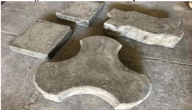
Fig. No. 7 Paver Blocks made up of CDW
