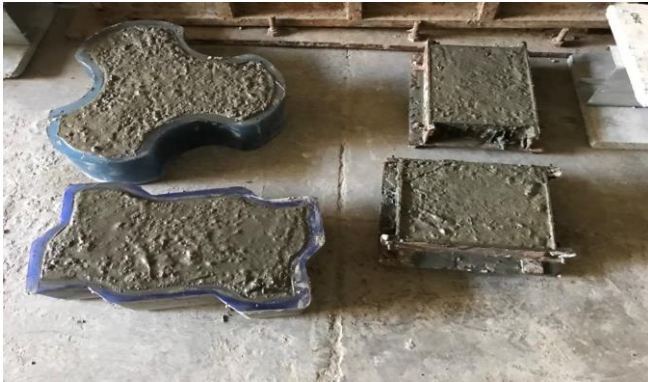
Fig. No. 7 Paver Blocks made up of CDW
