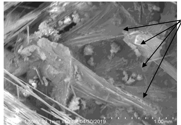
Figure 10: Position of sisal fibre in composite P1 after tensile test
