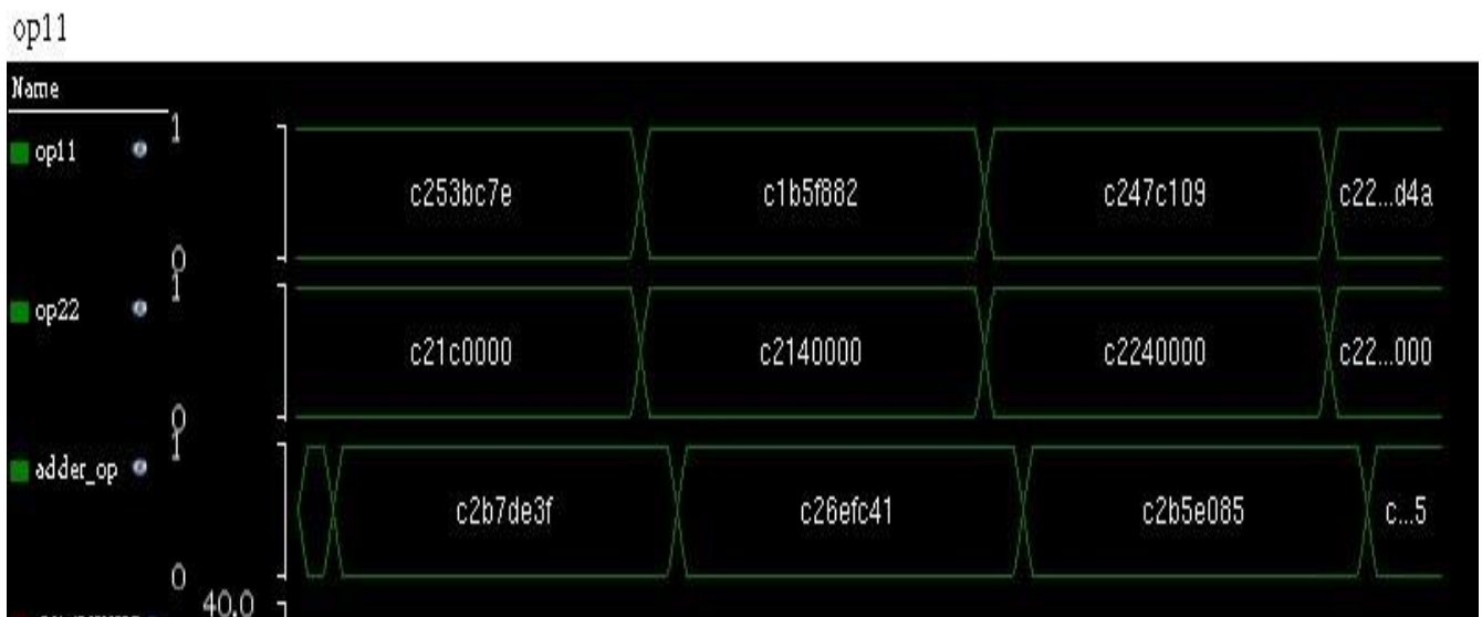
Figure 16: Simulation result for pipelined floating point adder/subtractor
