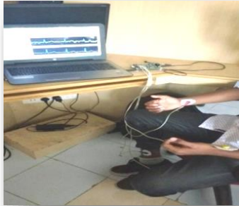
Figure 4 : 24-bit ECG acquisition (TI ADS 1293 EVM Board)
