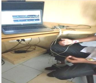
Figure 4 : 24-bit ECG acquisition (TI ADS 1293 EVM Board)
