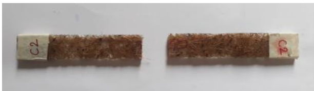
Fig.5: Specimens of Tensile Test After fracture
