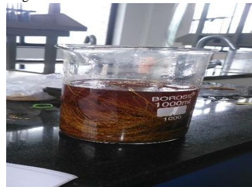
Fig. 1: Chemical Treatment of Coconut coir fibers with 2% NaOH
