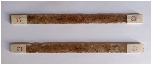
Fig.4: Specimens of Tensile Test before fracture
