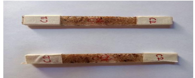
Fig. 7: Flexural Test Specimens Before Fracture
