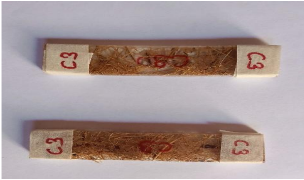
Fig. 10: Impact Test Specimens Before Fracture
