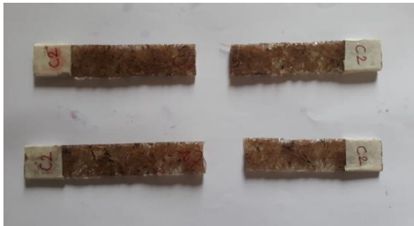
Fig. 11: Impact Test Specimens after Fracture
