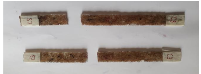
Fig. 8: Flexural Test Specimens After Fracture
