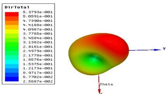
Figure 7: Radiation pattern in 3D of the Proposed Rectangular Micro-strip Patch Antenna
