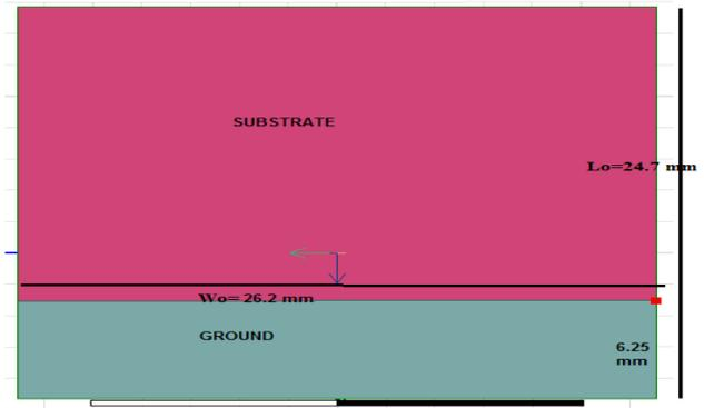
Figure 4: Back side view of patch
