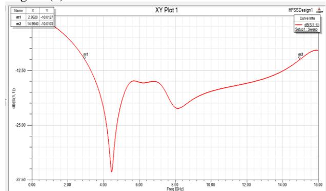
Figure 5: Return loss of the Proposed Rectangular Micro-strip Patch Antenna
