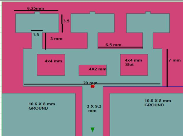
Figure 3: Front View of Rectangular Slotted patch-antenna
