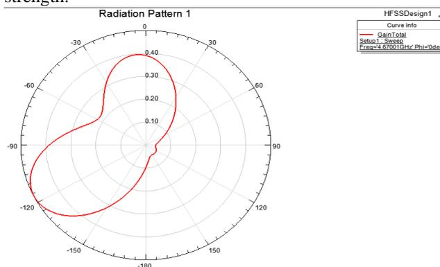
Figure 8: Radiation pattern in 3D of the Proposed Rectangular Micro-strip Patch Antenna
