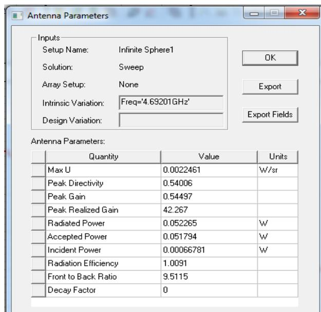
Figure 10: Parameter of Proposed Rectangular Micro-strip Patch Antenna
