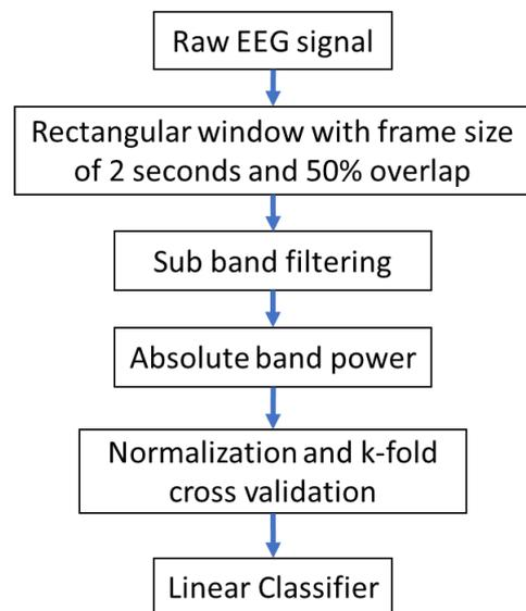
Figure 5. Flowchart of the signal processing
