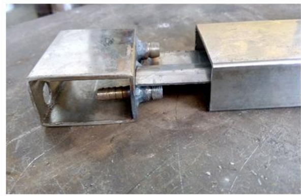
Fig. 6 Water inlet & outlet point
