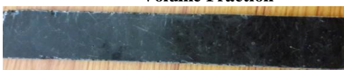
Fig.1.b Sisal Fiber and carbon nanotube reinforced Composite at 50% of fiber and 10% of CNT
