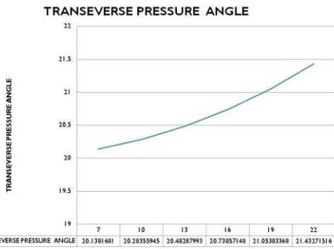
Figure 11 -Transverse Pressure Angle Vs Helix Angle The formula for the transverse pressure angle is given by following relationship-
