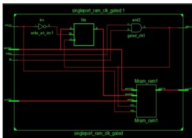
Figure 11: RTL implementation of single port RAM with clock gating
