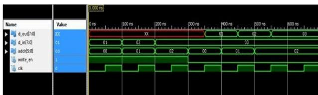
Figure 7: Simulation output of the single-port RAM
