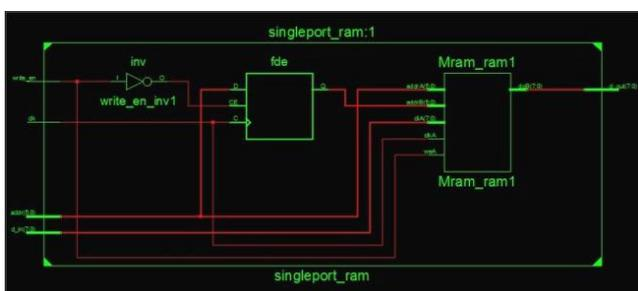
Figure 6: Detailed RTL implementation of single-port RAM
