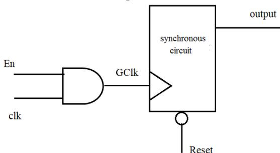
Figure 2: clock gating using AND gate
