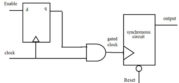
Figure 3: AND Gate Clock Gating Using A Latch
