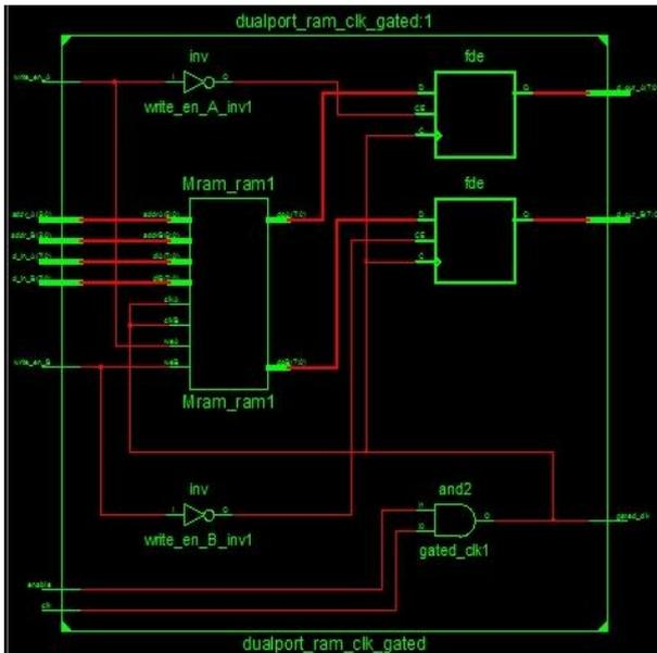
Figure 12: RTL implementation of dual port RAM with clock gating
