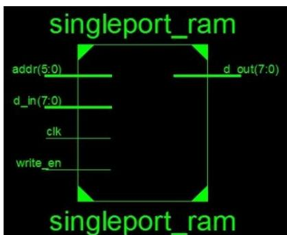
Figure 5: RTL schematic of single-port RAM
