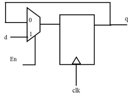
Figure 4: Multiplexer based clock gating
