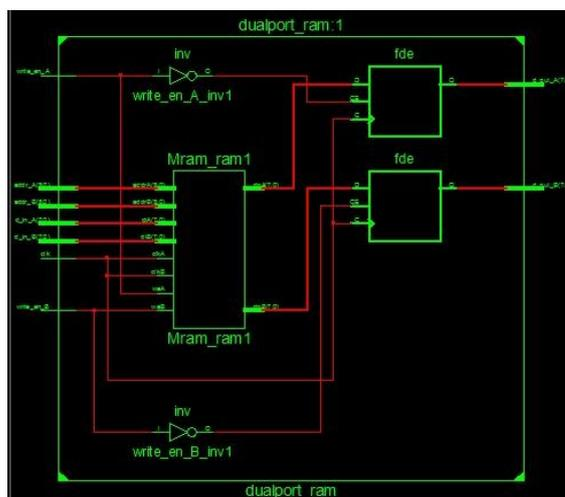
Figure 10: Detailed RTL schematic of dual port RAM
