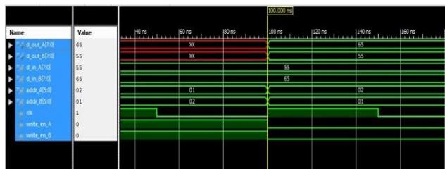
Figure 9: Simulation output of dual port RAM
