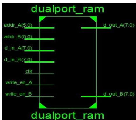
Figure 8: RTL schematic of dual port RAM
