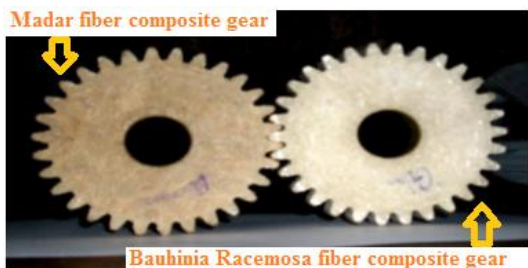
Fig.1 Madar and Bauhinia Racemosa composite gears
