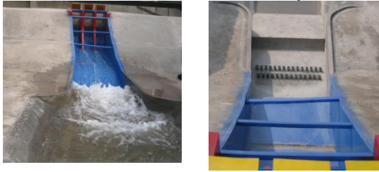
Fig. 1 Experimental set up of MyLam spillway and stilling basin
