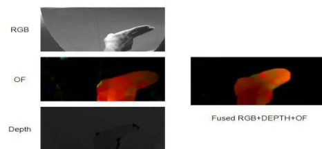
Fig. 4. Overall fusion after RGB, Depth and Optical flow, Strong response after assign more weight to optical flow.
