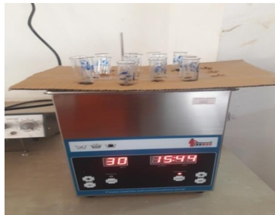
Fig 1: Ultra Sonication Of ZnO Nanoparticles
