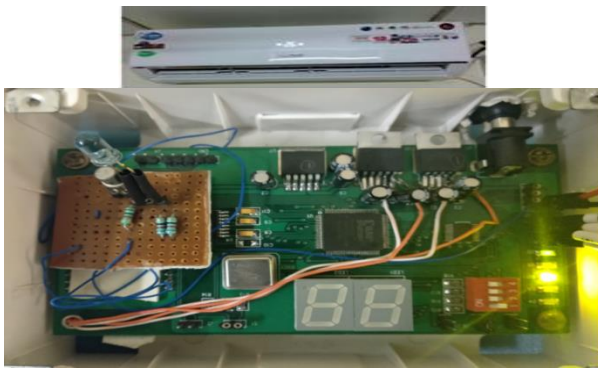
Fig.8. Hardware setup for 26°C AC power ON condition.
