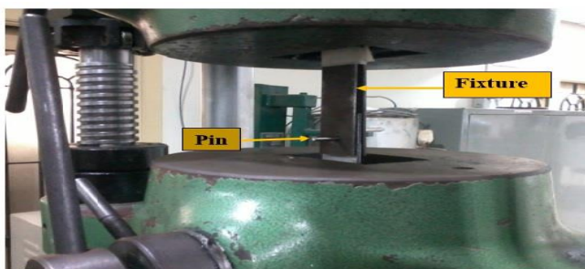
Fig.4. Bearing test on pin loaded CARALL specimens.
